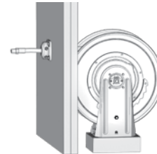
Truck Mount with Remote Mounted Roller Guide
