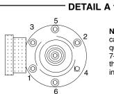
**NOTE:** Numbers indicate capscrew (4) tightening sequence. Torque evenly to 7-10 in-lb (0.8–1.1 N•m), then re-torque to 120-130 in-lb (13.6–14.7 N•m)
