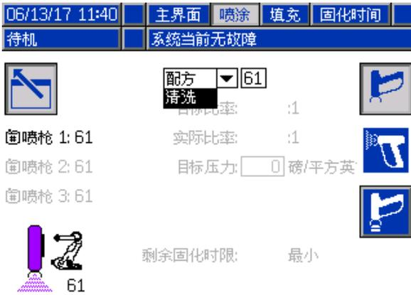
Figure 91 喷涂屏幕冲洗
