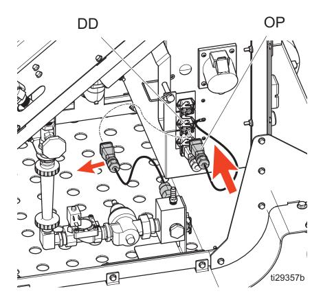
The water solenoid valve requires 40 psi of water pressure to be energized. If the water pressure is not 40 psi or greater, the solenoid valve will remain normally closed, blocking the flow of water. This operation can be overridden by unplugging the water pressure connector (DD) and connecting the water pressure override plug (OP). This mimics the signal that water pressure of 40 psi or greater is present, even when it is not.
