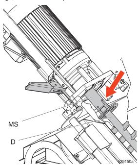
4. Swing the motor completely shut and lock it in place with the motor latch (K).
