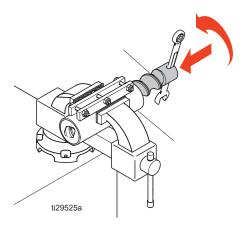
**NOTE:** Apply a lubricant to the rotor and stator beforehand to improve ease of assembly.
