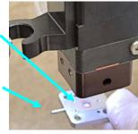
8. Tighten the two embedded screws with a 3-mm hex driver. Do not overtighten; it is possible to strip the screws. An optional torque wrench is available for this purpose (P/N NT09-2500).
