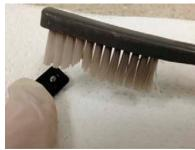
Figure 4-4 – Cleaning Brush (Advanjet P/N CLB-01)
