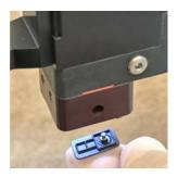
6. Note that the heater block has two pins that align with two holes in the nozzle plate.
