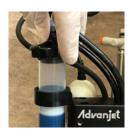
4. Attach a new feed tube to the luer (metal luer shown; selection of feed tube material depends on the dispensing fluid.
