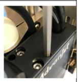
9. Before installing the fluid syringe, CLOSE the jet.
