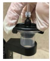
Figure 4-3: Replace Receiver Head
