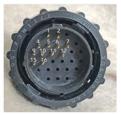
Figure 2-4: 28-Pin Jet Cable
