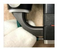
5. After the feed tube is in place, install the bottom half of the feed tube enclosure and tighten the setscrew.
