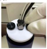
Lower the hot melt feed tube down into the melter so it extends out of the bottom.
