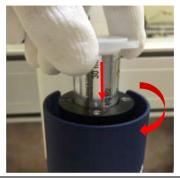
9. Replace the receiver head (top air supply) and tighten the thumbscrews.
