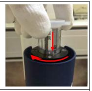
7. Use a <u>clean</u> probe tool to remove the layer of cured material from the top of the melted PUR.
