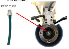
3. Pull down the end of the feed tube and jostle as needed until the luer is engaged in the bottom of the melter.
