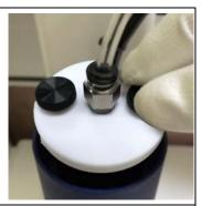
4. Turn the empty syringe counter-clockwise to disengage from feedtube luer lock, then pull it up and out.
