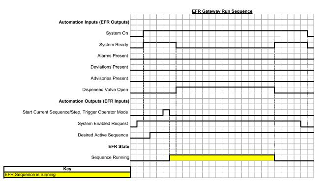
If the sequence is not in operator mode, a pulse on the Start Current Sequence/Step, Trigger Operator Mode bit will play the active sequence.
