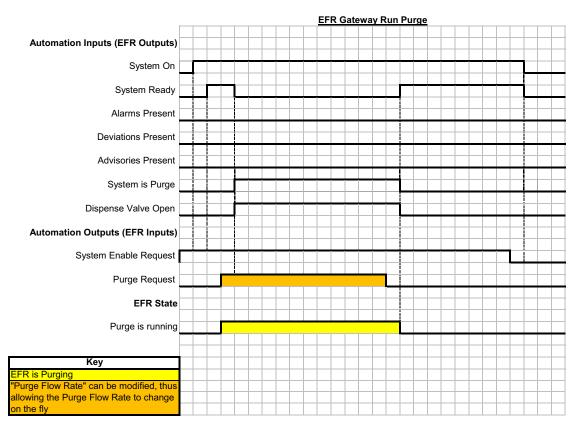
When the Purge Request bit is ON, the EFR will start purging as long as the System On bit is also ON. If the System On bit or the Purge Request bit is OFF, the EFR will stop purging.
