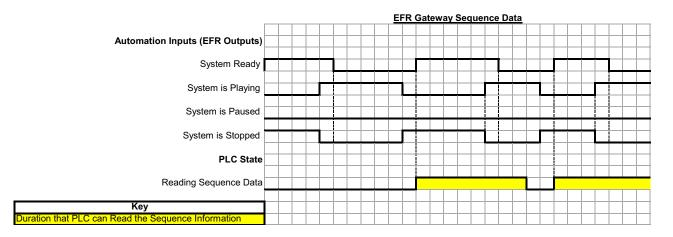
The Sequence Data must be read before the EFR finishes running another sequence. If the Sequence Data is not read before finishing the sequence, the data will be overwritten with new Sequence Data. The Sequence Data consists of:
