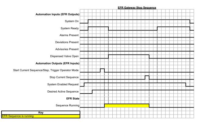
An ON pulse across the Stop Current Sequence bit will stop the active sequence.
