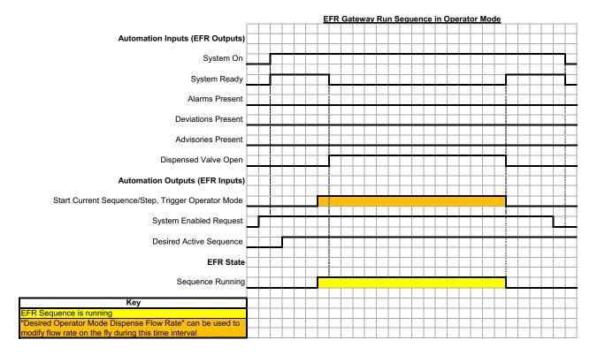
If there is a step in operator mode throughout the active sequence, the EFR will only dispense that step if the Start Current Sequence/Step, Trigger Operator Mode bit remains ON. Once the Start Current Sequence/Step, Trigger Operator Mode bit is OFF, the EFR will continue with the active sequence.
