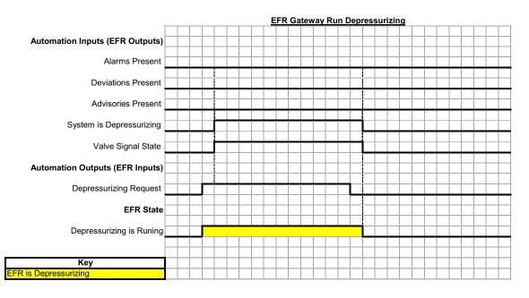
When the Depressurizing Request bit is ON, the EFR will start depressurizing. The EFR will only stop depressurizing if the Depressurizing Request bit if OFF.
