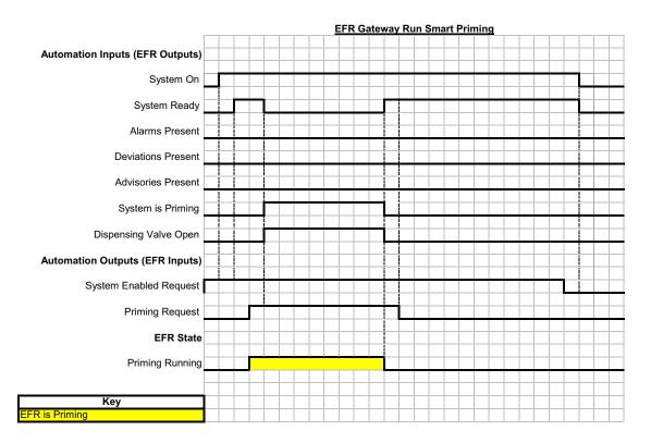
When the Priming Request bit is ON, the EFR will start priming as long as the System On bit is also ON. If the System On bit or the Priming Request bit is OFF, the EFR will stop priming.
