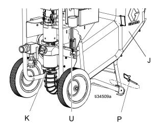
3. Remove the locking pin and pull down the hopper latch (U) on the hopper plate.
