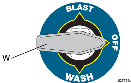
FIG. 1: Turn the Selector Valve Off
