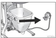
Place Drain Tube in waste bucket. For disinfectants with alcohol active ingredients, ground the bucket according to **Grounding**, page 10.
