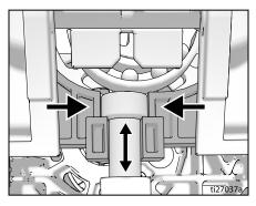
Swing Easy Access Door pump door closed while pushing the entire door towards the inlet end of the pump.
