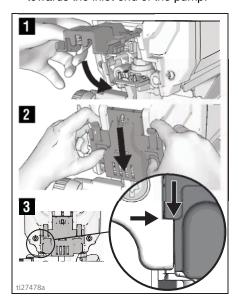
**NOTE:** Door must be fully closed and latched before sprayer will operate.
