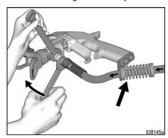
4. Remove Spray Tip Guard assembly from Spray Gun.
