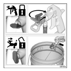
Engage Trigger Lock. Rotate Spray Tip back to SPRAY position. Disengage Trigger Lock and continue spraying.
