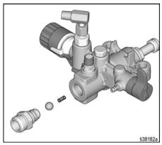
Clean any debris from the cavity and reinstall the ball and spring. Tighten inlet valve to pump using integrated tool on the frame.
