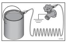
To maintain ground continuity when sprayer is flushed or pressure is relieved: Hold metal part of Spray Gun firmly to the side of a grounded metal pail then trigger the Spray Gun.
