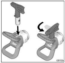
4. Screw Spray Tip Guard assembly onto Spray Gun and tighten.
