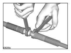
Insert other end of Airless Whip Hose through Hose Guard at base of Spray Gun. Connect to Spray Gun. Use wrenches to tighten securely.
