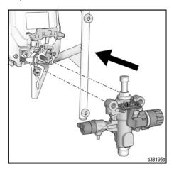
2. Move pump displacement rod up or down until cap is level with the opening in the yoke.
