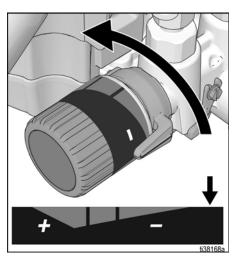
4. Put Drain Tube in a pail and turn Prime/Spray Valve horizontal to PRIME position to relieve pressure.
