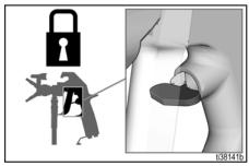
Turn Prime/Spray Valve horizontal to PRIME position.
