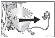
While holding the Drain Tube retainer with the Drain Tube parallel to the top of a waste bucket, twist retainer over the lip of the container. Drain Tube should now be inside the waste bucket.
