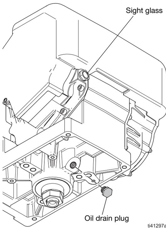
**FIG. 15 Oil drain plug**
