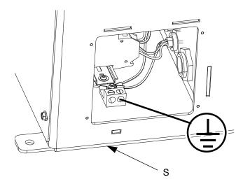
Fig. 8: Attach Ground Wire
