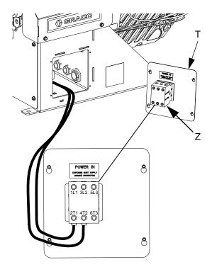
Fig. 7: Terminal Connections
