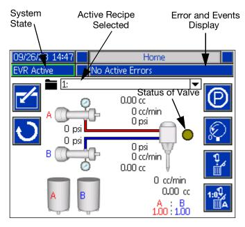
The home screen is the first screen displayed when the ADM is turned on. Here you can monitor the actual flow rate, actual amount dispense, and the current fluid pressure on the A and B fluid outlets of the pump. If installed, the inlet pressure of the pump will be displayed. Note: While the machine is in dispense mode, the system will show actual ratio in the bottom right hand corner instead of the set point.
