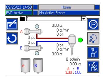
**Purge:** When pressed, the purge icon will purae material from the pumps. To stop purging material from
