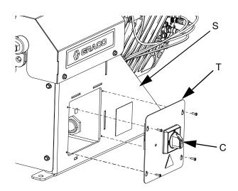
Fig. 6: Remove EVR Frame Cover
