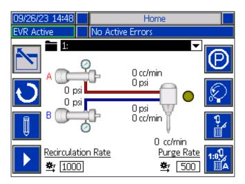
To select a recipe, use the navigation keys to highlight the active recipe bar. Then press the Enter button
