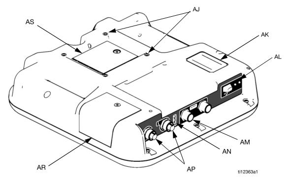
Fig. 4: ADM Component Identification - Rear
