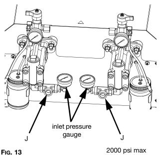
Ensure the supply systems and, if applicable, the inlet regulators are off or set to zero pressure before connecting.
