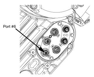
Fig. 12: Electric Driver Port #6
