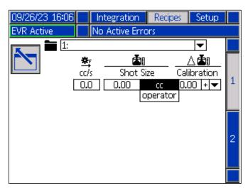
**NOTE:** If the user selects operator mode for the shot size, the EVR will only dispense at the desired flow rate as long as an external trigger source or foot switch is active for that particular shot of the recipe.
