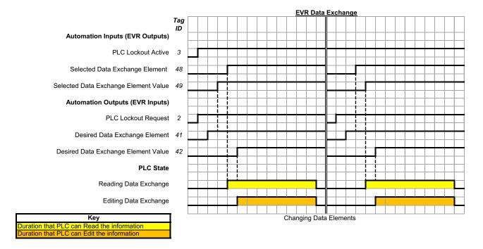
**NOTE:** PLC lockout has to be enabled to write a data exchange element value. To request a data exchange element, the PLC lockout does not have to be enabled.
