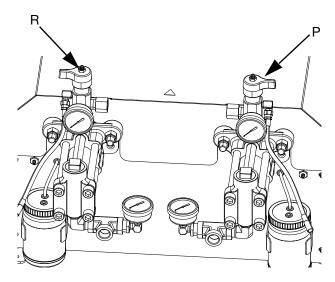
4. For models with a dispense valve with a safety lock, engage the dispense valve safety lock.
