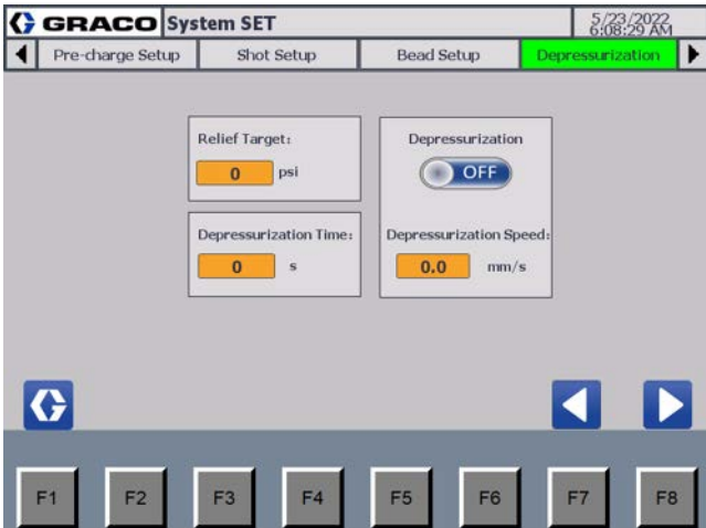
FIG. 26 De-pressurization Setup Screen
